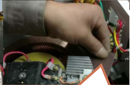
Figure 3: put the opposite of sandpaper on the surface of coil, use hand to lift the carbon brush, then release to press the sandpaper, carbon brush pull the sandpaper back and forth or swing the carbon brush back and forth about 5-6 times, let it contact with coil fully.
